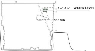
Place the Skimmer enclosure into the excavated hole. Check the top of the enclosure to make sure that it is level front-to-back and side-to-side. Check where your pre-determined water level falls on the face of the Skimmer enclosure. The water level needs to be between 11/4" and 11/2" below the top of the weir door opening and/or even with the water level indicator molded on the side of the Skimmer.
