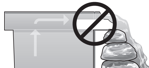
Ex. 9 If using a natural rock for your waterfall lip, make sure that it is fairly thin. (no more than 3/4")
